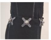
2. Ensure that the foot markers are placed so that the toe marker is as far forward as possible on the foot while still facing upward. Also ensure that the three other markers (the heel marker and the two markers on either side of the front of the foot) are in the same plane, and are as low (ie near to the floor), as possible.
