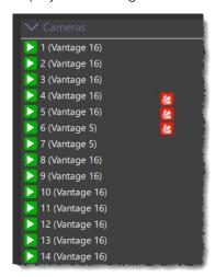
To prevent you from having to recalibrate the whole system after a camera has received a minor bump, when a calibrated subject (or prop, or wand) moves through the volume, cameras automatically detect whether further action is necessary:
