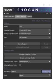
A single-segment prop is created from the selected markers and appears in the **3D Scene** in the orientation defined by the order in which you selected the markers in the previous step.
