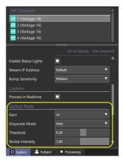
When you have finished focusing and optimizing the cameras, with all cameras selected, in the **Optical Mode** section change **Grayscale Mode** back to **Auto**.
