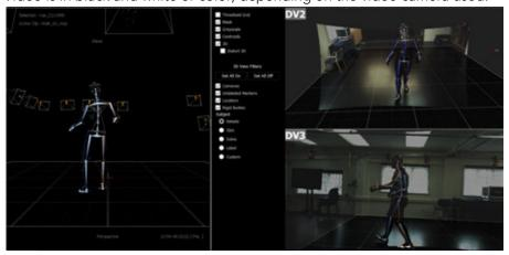
8. To see the image plane of the camera corrected for lens distortion, select **Distort 3D**.
