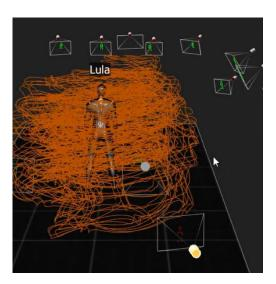
4. When enough of the view has been covered (indicated by orange trails that thickly cover the affected camera view, as shown above), click **Recover Camera Position** again.
