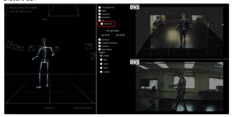
The 3D overlay should line up with the subject in the **Cameras** view and the grid should line up with the floor.
