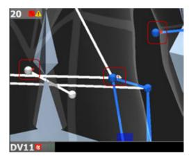
Shogun Live enables you to quickly correct a camera whose position has changed due to having been bumped or moved, using any labeled object in the volume – subject, prop, or wand, and the Recover Camera Position feature.
