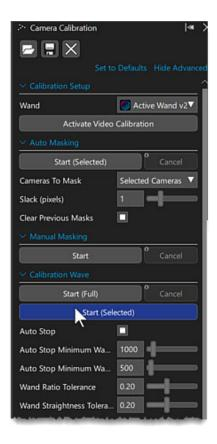
In the volume, ensure that the person waving the wand does not stand too close to the new or moved camera, so that the wave can be captured by both the directly affected camera and the adjacent cameras.
