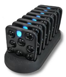
The average battery run-time for a Pulsar used at 100% brightness is around nine hours of continuous use. You can extend battery life by disabling Pulsars when not required for tracking, which will give up to 18 hours of typical use.
