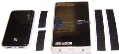
3. Attach the two 60mm strips of hook tape widthways to the Power Pack, 4.5cm apart (so you can later attach it to the long strips on the rods).
