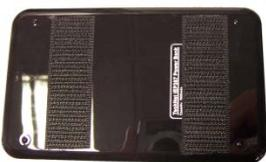
4. Attach the two 130mm strips of hook tape 4.5cm apart lengthways along the HDMI receiver.
