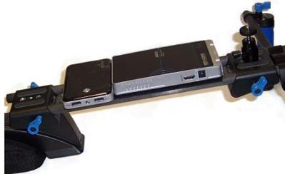
7. Remove the field monitor from its box and attach it to the monitor mount that you previously fitted.
