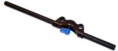
7. Loosen the blue locking screws on the handgrips, slide them onto the short rods and re-tighten the screws.
